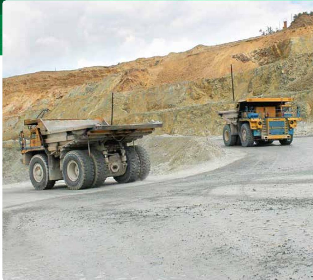
slower evaporation of water, increased ground moisture, better surface compaction with less surface deterioration. Therefore there are no potholes and rutting creating dust and the surface keeps its optimal condition.
